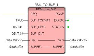
Setting BUF\_FORMAT to TRUE will ensure that the Android App properly interprets the input
