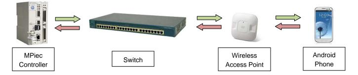
Of course this is a fairly simplified network diagram but the idea is correct. One could also connect to a controller remotely but that would involve configuring VPN access on the Android phone.
