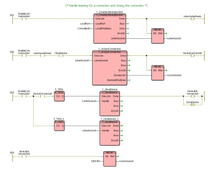
This methodology allows a single connection to be opened to the controller from a requester over port 23. It is important to note that the port number is independent of the application – you can choose the port number your controller and Android device communicate over, however it is suggested to avoid common port numbers associated with services like FTP, SMTP, etc. The above IEC code also handles a commanded disconnect that
