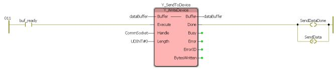
This same sort of communication methodology can be expanded and enhanced to receive and send significantly more complicated packet structures allowing large amounts of control and data gathering with a fairly simple set of function blocks and a custom command processing function block.
